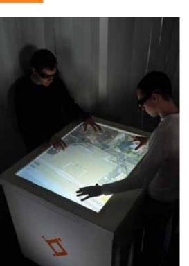
The Map Table is a revolutionnary multitouch, multiuser, stereoscopic device developed by Immersion. It allows both the 3D visualization and interaction with the geospatial environment displayed by the Explorer.
